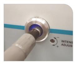
Figure 1. Insert Lightguide into Lightguide Mount
