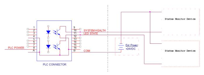
For sinking current below 7mA it is suggested when using solid state relays to use one of these devices: Weidmuller 8820710000, Phoenix Contact 2980636.
