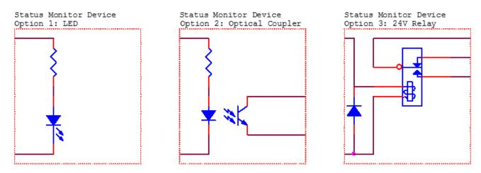
PLC Power channel is a 24V source available for use to drive PLC logic but must be current limited using pull-down resistors to protect the BlueWave AX-550 V2.0 when directly attached to the I/O channels through the PLC connector.
