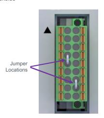
**Figure 14.**PLC Connector Pin Map with Jumper locations highlighted
