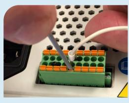
**Figure 11.** Remove Jumper from Terminal Block
