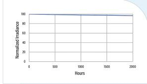
Figure 7. LED Degration Testing - VisiCure®
