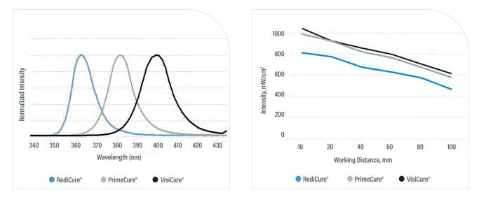
Figure 2. BlueWave® AX-550 V2.0 Emitter Spectral Output Chart
