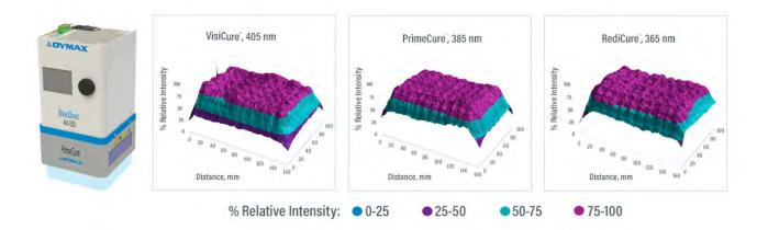
NOTE: Curing area data taken using Fuji UV Light Distribution Mapping System. Output intensity normalized using a Dymax ACCU-CAL<sup>™</sup> 50-LED Radiometer.
