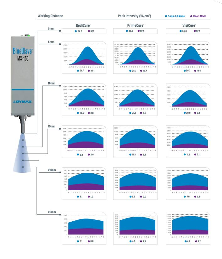
\* Dymax recommends using the 5-mm lightguide source mode on the ACCU-CAL<sup>™</sup> 50-LED, when measuring at 0 mm with the provided adapter in the ACCU-CAL kit. If measurements are made at greater working distance, Dymax recommends using the flood mode source for measurements. For convenience, both numbers are provided in this chart.
