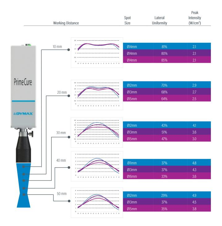
\* Dymax recommends using the flood mode source for measurements. The units of the X-axis in the charts are millimeters (mm). The spot size varies with both the distance of the emitter and the focus change of the lens. By referring this chart, the best combination of spot size, uniformity and intensity can be obtained by adjusting the emitter distance and focus of the lens.
