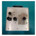
Figure 6. Bypass Connectors Installed
