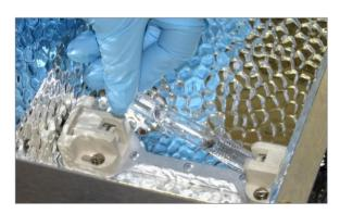
Step 6. Install the new bulb by following Steps 4 & 5 in the reverse order.
