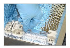
Figure 11. Lift Bulb
