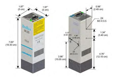
When multiple emitters are mounted side-by-side, maintain 1 mm (0.04") of clear space between units. For outermost units, maintain 20 mm (0.8") of free space to obstructions for safe use.
