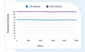
Figure 6. LED Degration Testing - VisiCure
