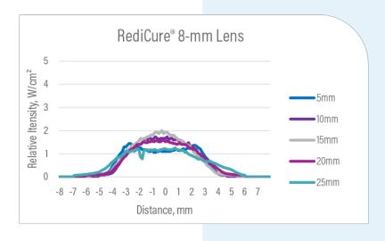
Note: Curing area data taken using Fuji UV Light Distribution Mapping System and normalized to ACCU-CAL™ 50 LED Radiometer.
