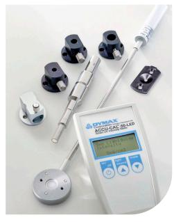
ACCU-CAL<sup>™</sup> 50-LED for measuring LED spots and flood lamps PN 40505
