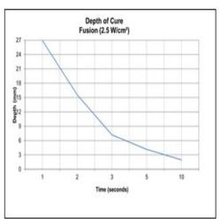
B Intensity was measured over the UVA range (320-395 nm) using a Dymax ACCU-CAL™ 160 Radiometer.
