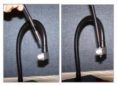
Figure 2. Insert Lightguide into Lightguide Holder
