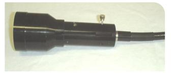
Gently tighten the knob on the end of the rod lens to secure the 8-mm lightguide to the lens. This completes the installation.
