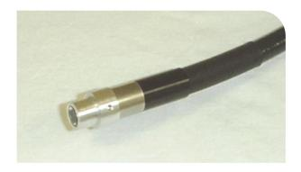
2. Place the adapter on the end of the 8-mm lightguide & gently tighten the setscrew.
