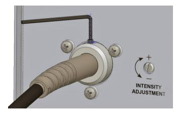
If desired, the Lightguide may be fastened into place by lightly tightening the Securing Set Screw in the top of the Lightguide Mount. A Hex Wrench is provided with the unit for this purpose. The Set Screw should be tightened gently to prevent damaging the Lightguide.
