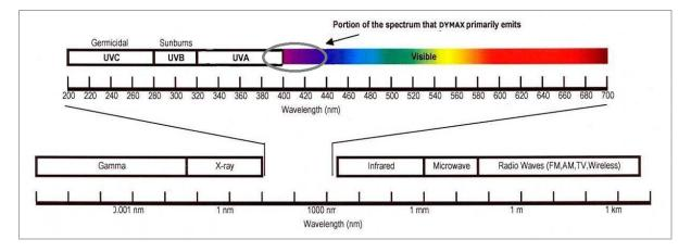
Standard Dymax VisiCure systems have been designed to primarily emit visible light (as shown in Figure 1). Although OSHA does not currently regulate visible or ultraviolet-light exposure in the workplace, the American
