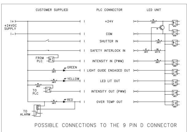
Figure 9. 9-Pin D Connector I/O Signals
