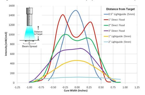
Figure 17. BlueWave<sup>®</sup> LED DX-1000 Intensity by Distance and Delivery Mode
