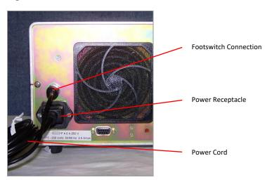
Figure 3. Cable Connection, BlueWave 200 Rear Panel
