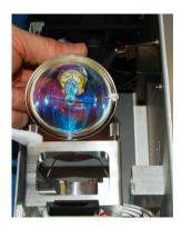
4. Unpack the new Bulb. Take care not to bend the flat Electrode in the center of the Bulb.
