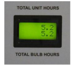
**WARNING!** Operating a BlueWave 200 Lamp beyond 2,000 hours will result in a non-passive failure of the lamp! Do not reset the Lamp Dual-Hour Meter without replacing the bulb.
