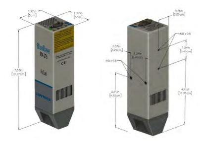
When mounting multiple emitters side-by-side (Figure 3) maintain 1 mm (0.04") of clear space between units. The outermost units must have 20 mm (0.8") clear space from obstructions for safe use.
