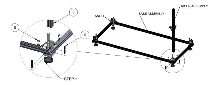
Figure 4. Attach the Riser Assemblies to the Base Assembly
