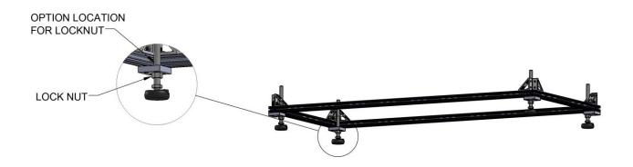
Figure 3. Optional Location for Locknut For Conveyors with a Chain-to-Floor Height of 35.6" (905 mm) or Less
