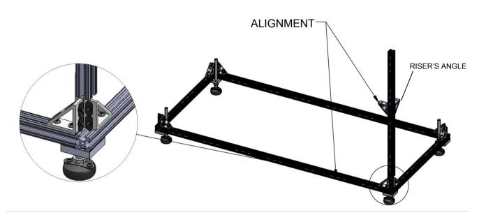
Figure 5. Correct Alignment for Riser Assembly
