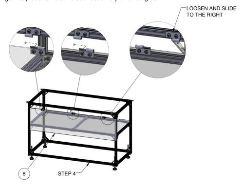
Figure 8 Loosen the hinges
