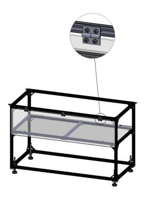
Figure 9. Door Assembly Attached
