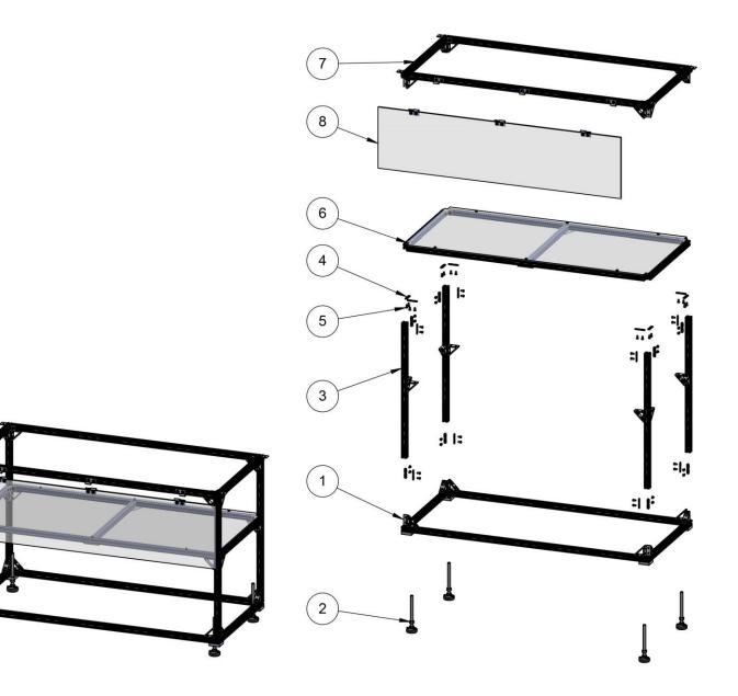
Figure 1. Cart, Exploded View
