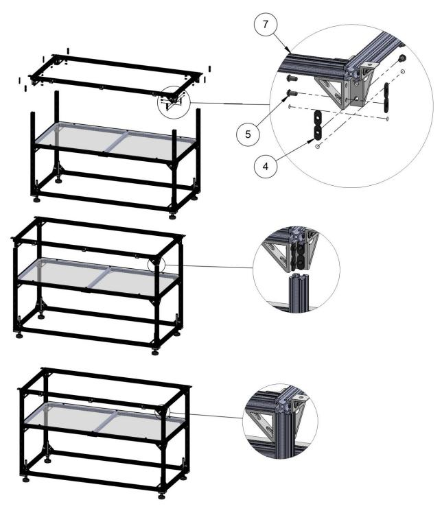
Figure 7. Attach Top Assembly
