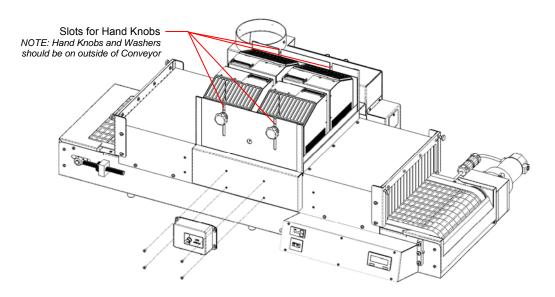
Figure 12. Install Cradle and Switchbox
