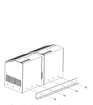
Figure 9. Mount Remaining Arrays on Cradel Adapter
