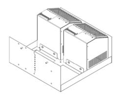
Figure 8. First Two LED Arrays Mounted in Cradle
