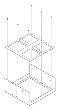
Figure 5. Attach the Cradle Adapter (41988) to Cradle (41989)
