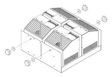
Figure 11. Loosely Install Hand Knobs and Washers on Cradle
