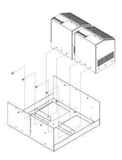
Figure 7. Mount LED Arrays in Cradle with M5 x 8-mm Screws
