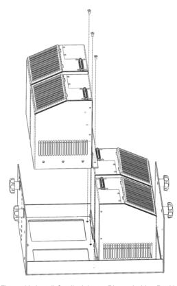
Figure 10. Install Cradle Adapter Plates, In-Line Position
