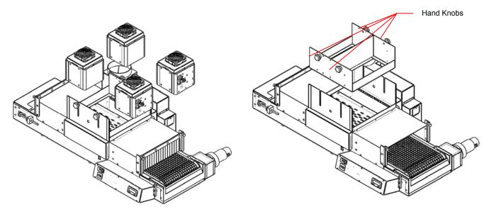
Figure 2. Remove Reflectors
