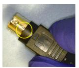
Position of plastic when housing is not retracted
