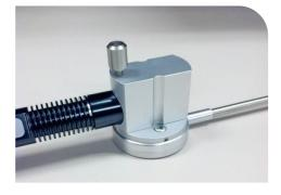
4. Press and release the On/Off button on the radiometer's face plate to turn the unit on.
