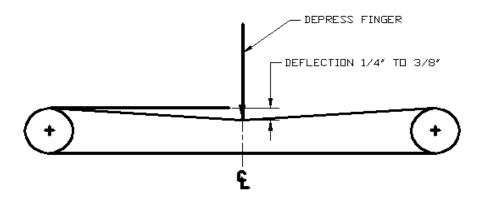
Dymax recommends that the Curtain Drive-Belt's tension be checked at least once every three months. Follow the instructions below to check the tension.
