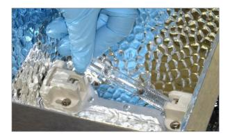
Step 6. Install the new bulb by following Steps 4 & 5 in the reverse order.
