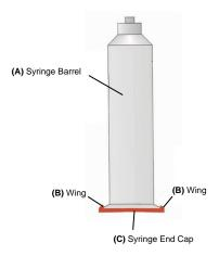
**Figure 2.** Micro-Dot Component Diagram
