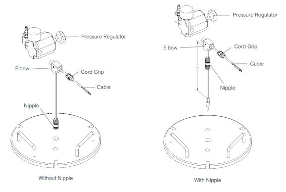
5. Assemble the Regulator, Tee, and Cord Grip (and Nipple) together in the orientation shown in Figure 12. Ensure that the pipe threads are tight.
