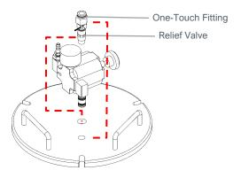
2. Remove the Pressure Regulator Assembly (Figure 9). If the Nipple stays on the Lid, use the figures on the left for reference. If the Nipple comes off with the Regulator, use the figures on the right for reference. Kit T18500 comes with an additional Nipple.
