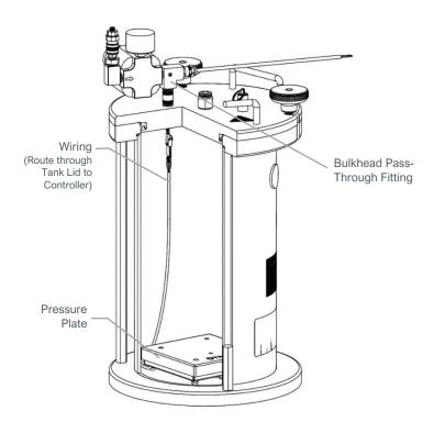
Strip the 1/4" wire ends and secure the connections to the SB-100 Controller. Ensure the Pressure Plate Sensor Connections are secure. (See SB-100 Controller Setup, page 17) 4. Connect the Power Jack, Beacon, and any external controls to the SB-100 Terminal Connections. (See SB-100 Controller Setup, page 17)
