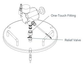
7. Install the Lid on the Tank with the Pressure Plate Sensor. Adjust the cable length inside the Tank so the Lid can be removed and placed next to the Tank without moving the Pressure Plate Sensor. Tighten the Nut on the Cord Grip. Do NOT over tighten. Install the Lid again and pressurize the Tank to inspect for air leaks. It is normal for the Pressure Regulator to bleed a small amount of air when pressurized.
