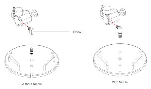
4. Remove any old Teflon off the pipe threads and apply Teflon tape to all pipe threads. **Do NOT** apply Teflon tape to the Cord Grip. Feed the Cable through the Nipple, Tee, and Cord Grip as shown in Figure 11. Note that the Connector does NOT fit through the Nipple. Do NOT tighten the Cord Grip.
