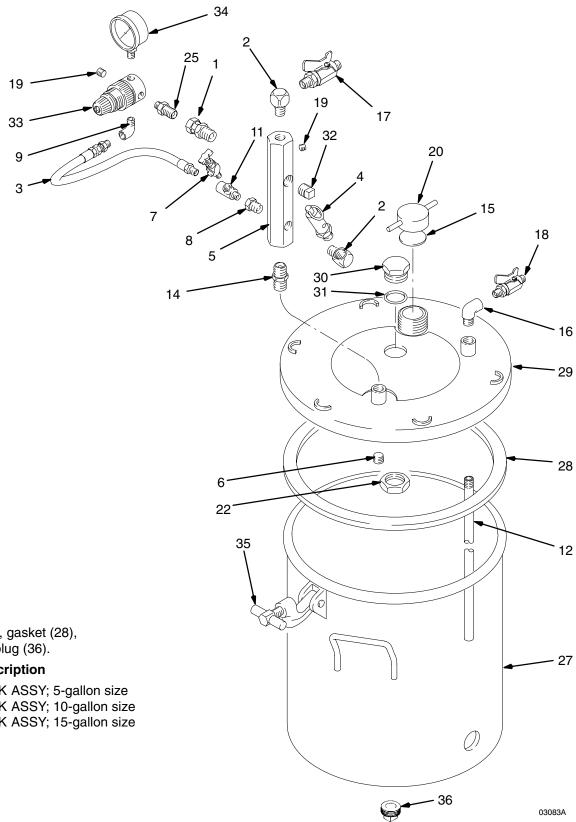
Tank Assemblies include tank (27), gasket (28), cover (29), and plug (36).
