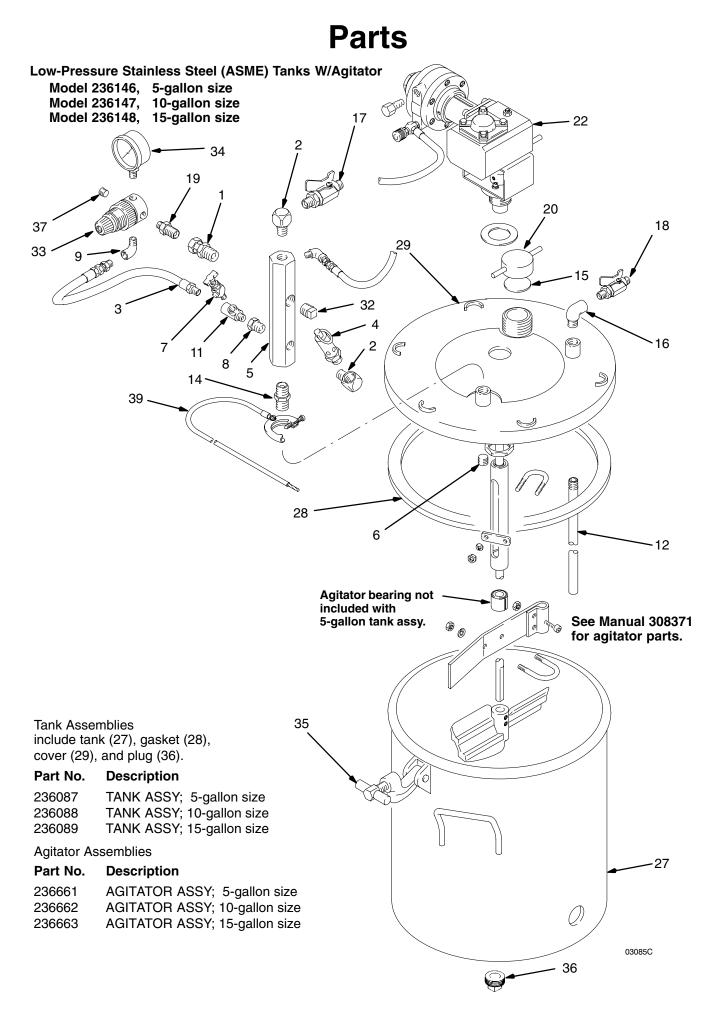
Low-Pressure Stainless Steel (ASME) Tanks W/Agitator
