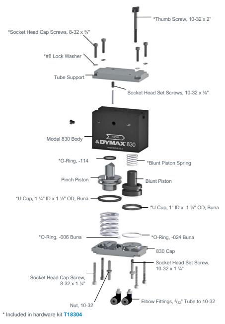
Figure 14. Tubing Assembly
