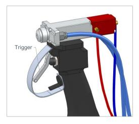
6. Adjust the pressure on the atomizing air regulator (Figure 12) between 2-3 psi (0.14 - 0.21 bar) for startup.
