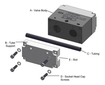
*Note:* The Model 828 is not supplied with tubing. Various tubing sizes and materials (including polyethylene, polyurethane, PVC, and silicone) are available for order through Dymax. This valve is compatible with a maximum tubing size of 0.375" [9.53 mm] OD.
