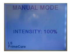
**NOTE:** If your unit doesn't display the 'LS' symbol on the screen, remove all power and do not operate the unit. Contact Dymax for assistance.
