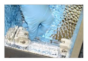
Figure 11. Lift Bulb
