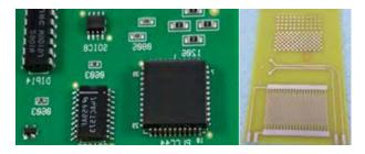
A humidity chamber was set to 85°C, 85% RH for 2,000 hours to evaluate heat and humidity resistance of the coatings. Salt spray corrosion resistance was evaluated using ASTM B117.
